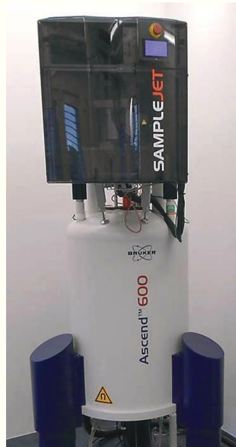
Figure 3: 600 MHz NMR spectrometer with auto sampler. Fully automated processing and evaluation of samples offers up to 29 parameters for optimal judgement of a potential risk of myocardial infarction.
